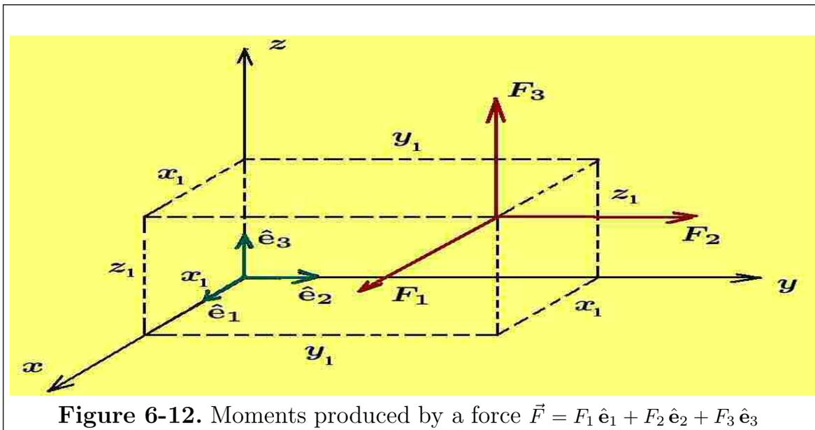
Figure 6-12. Moments produced by a force  $\vec{F} = F_1 \hat{e}_1 + F_2 \hat{e}_2 + F_3 \hat{e}_3$
