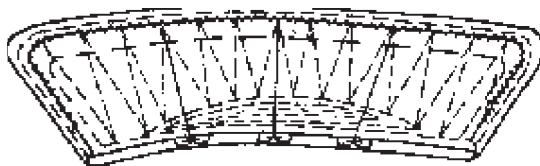
4.47-rasm. Ustki yoqani ostki yoqaga yashirin siniq baxyali maxsus mashinada bostirib tikish.
